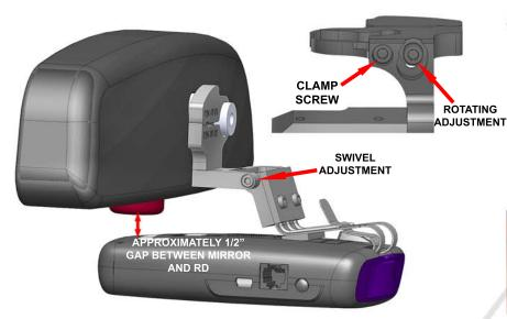
5 - Install the RD onto the mount. Make the necessary adjustments as shown above. Using the vertical adjustment, we recommend you adjust the RD so there is approximately 1/2" gap between the bottom of the mirror and the top of the RD. After all adjustments are made, be sure to check that all adjustment screws are tight. Grab the long arm of the allen wrench to assure that these screws are securely tightened. You will not strip out the tapped holes in the aircraft grade aluminum.
