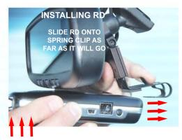
7 - When removing or installing the RD, squeeze the trigger and the back side of the mount together with one hand, and lift the front of the RD upward with the other hand before sliding the RD off or onto the spring clip. You must lift the front of the RD upward before sliding it off or onto the mount.
