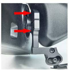
4 - Position the mount as far forward as you can. Before fully tightening the clamp screw, make sure the bottom of the mount is parallel with the bottom of the mirror.
